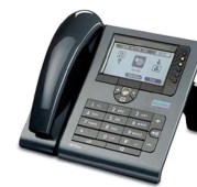
Netfon 500 LAN telephone set with integrated 2 port 10/100Tx switch
