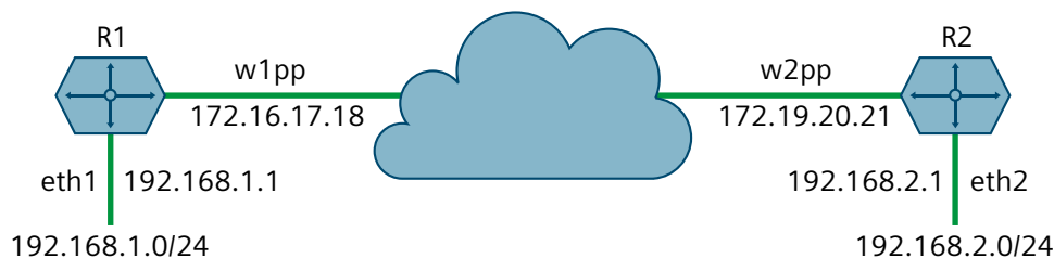
Figure 19: Example – GRE Tunnel Configuration
